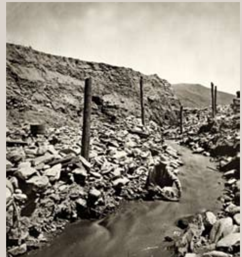
FIGURE 6.21: Gold panning was the simplest way to remove loose gold dust and nuggets from a streambed.
