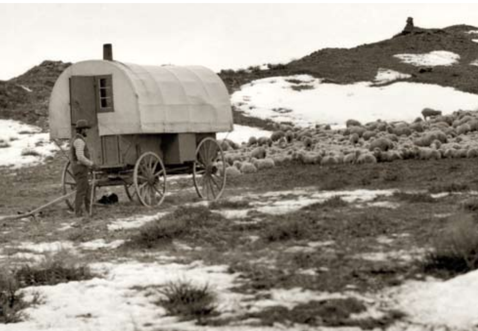
FIGURE 8.10: Shepherders tended their flocks all winter. They cooked, slept, and stayed warm in sheep wagons with multilayered canvas tops. Inside was a stove, dish cupboard, storage cupboard, bench, and bed. When it was time to move the flock to new grazing ground, the herder hitched the wagon to a team of horses and moved camp.
