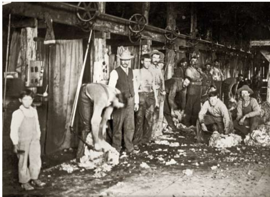
FIGURE 8.11: Shearing time was a period of sweaty, backbreaking work for the shearers. Rancher George Burt (in the black vest) was one of the first to try mechanical shearing. Note the power shears hanging from wheels at each shearer’s stall.
